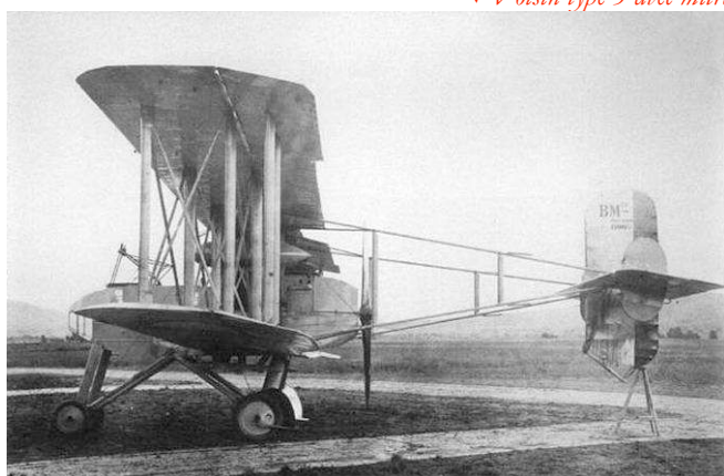
Bréguet-Michelin B2, 1916 (hélice propulsive) ↑
